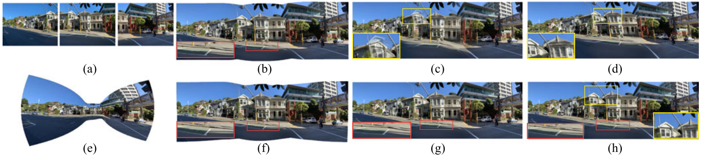
Fig. 4. Ablation study of our energy terms for rectangular stitching. (a) input images, (b) initial stitching result, (c, d, g) stitching results obtained by removing \phi_a , \phi_s , \phi_r , and \phi_l respectively, (e) initial stitching result with a very small weight for \phi_\rho as no result is produced without this term, (h) our stitching result using all energy terms.
